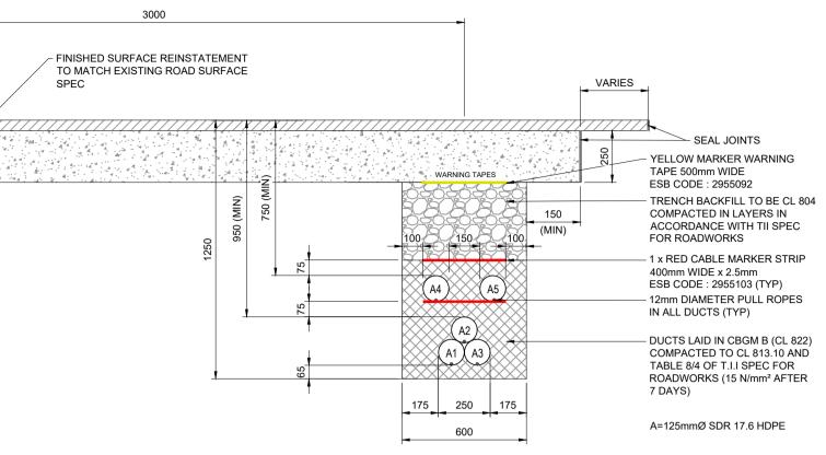
CARRIAGEWAY REINSTATEMENT TRENCH FOR 125mm DUCTS IN TREFOIL SCALE 1:20
